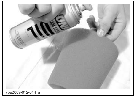
TYPICAL - OIL THE FOAM FILTER ELEMENT
