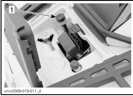
TYPICAL — SERVICE COMPARTMENT 1. Reservoir
