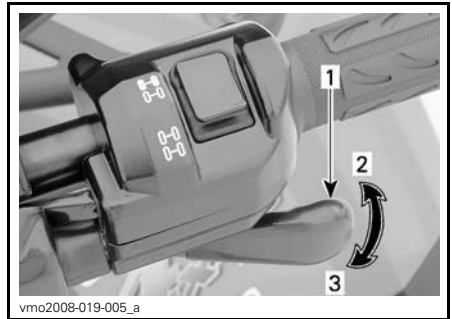
TYPICAL 1. Throttle lever 2. To accelerate 3. To decelerate
