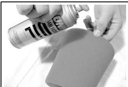
TYPICAL - OIL THE FOAM FILTER ELEMENT
