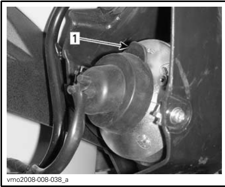
REMOVE RUBBER PROTECTOR 1. Rubber protector
