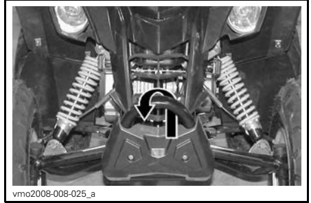
DS 90 — FRONT TIE-DOWN POINT LOCATION
