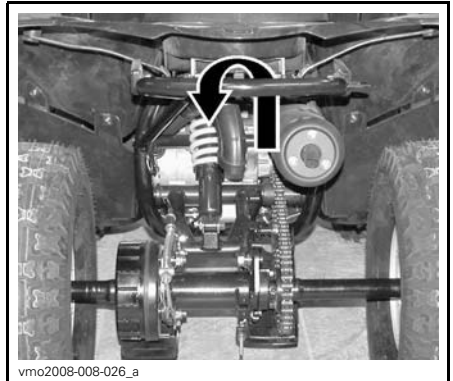
ALL MODELS — REAR TIE-DOWN POINT LOCATION
