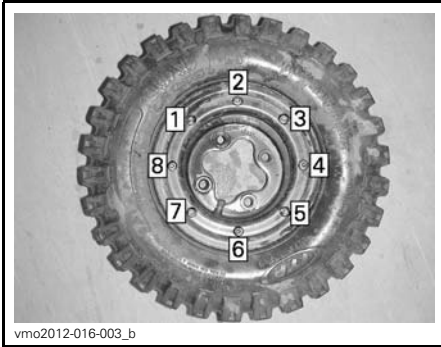
8-BOLT BEADLOCK WHEELS — FINAL STEP TIGHTENING SEQUENCE
