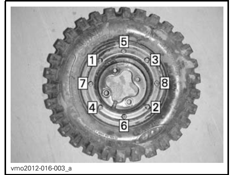
8-BOLT BEADLOCK WHEELS — FIRST AND SECOND STEPS TIGHTENING SEQUENCE
