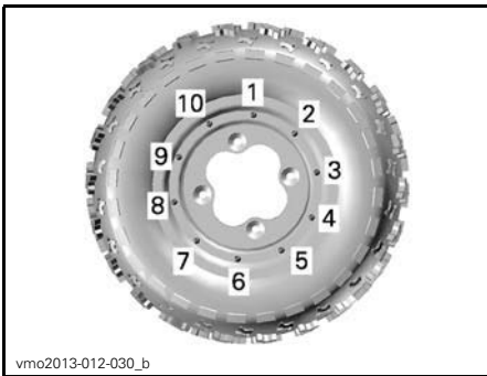
10-BOLT BEADLOCK WHEELS — FINAL STEP TIGHTENING SEQUENCE
