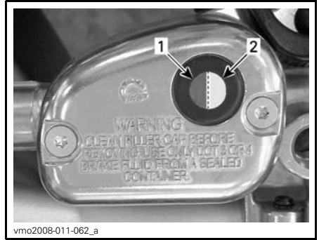
TYPICAL 1. Proper fluid level 2. Low fluid level
