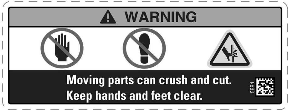
IBR GATE - WARNING LABEL
