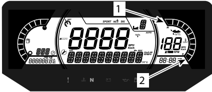
TYPICAL – INFORMATION CENTER – VTS POSITION INDICATOR
