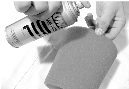
TYPICAL - OIL FOAM FILTER ELEMENT
