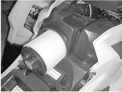
AIR FILTER REMOVAL
