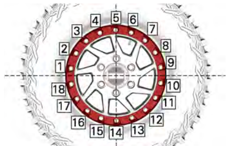
TYPICAL - FINAL TIGHTENING SEQUENCE
