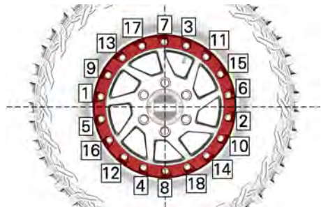
TYPICAL - TIGHTENING SEQUENCE
