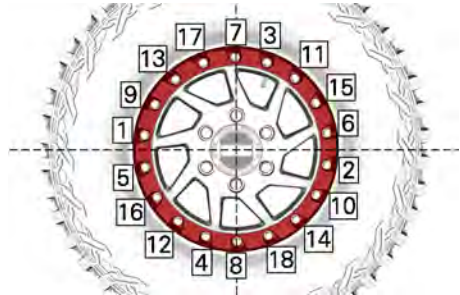
TYPICAL - TIGHTENING SEQUENCE
