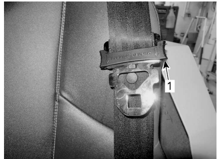
TYPICAL - LOCKED POSITION
