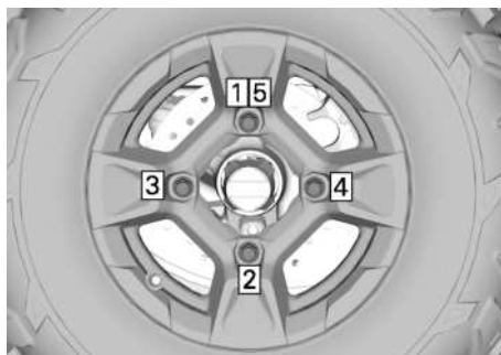
TIGHTENING SEQUENCE
