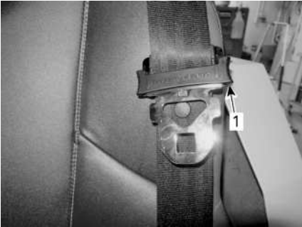
TYPICAL - LOCKED POSITION
