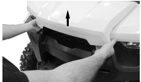
LIFTING FRONT SERVICE COVER EDGE.
