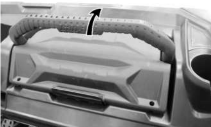
SECURING TOOL BOX IN PLACE
