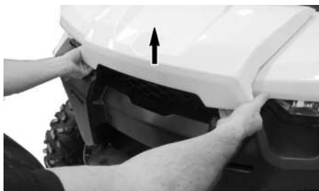
LIFTING FRONT SERVICE COVER EDGE.
