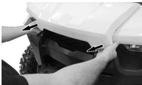
PULLING ON FRONT SERVICE COVER EDGE.
