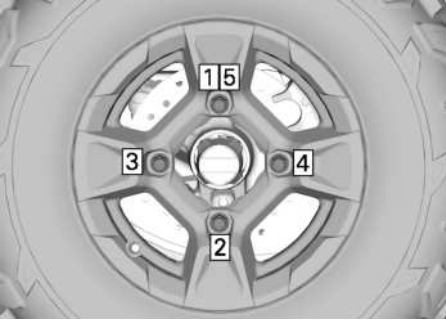
TIGHTENING SEQUENCE
