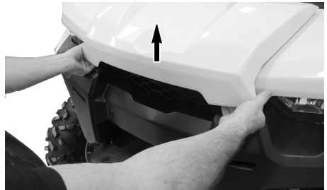
LIFTING FRONT SERVICE COVER EDGE.
