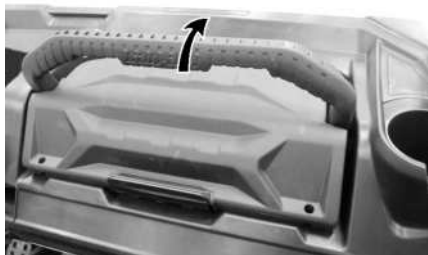
SECURING TOOL BOX IN PLACE
