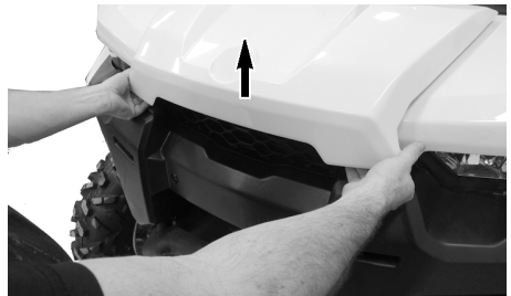
LIFTING FRONT SERVICE COVER EDGE.
