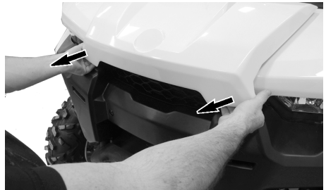
PULLING ON FRONT SERVICE COVER EDGE.
