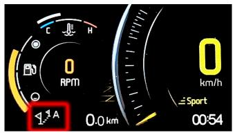
Repeatedly depress the HI/LOW beam switch rapidly, then, while doing this, press and hold the Volume Down/ Cancelling Call button until the following message appears on the display.
