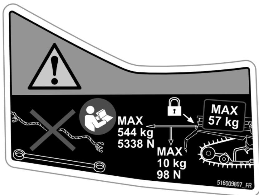
CHARGE CARGO MAXIMALE ET CAPACITÉ DE REMORQUAGE - ÉTIQUETTE D'AVERTISSEMENT
