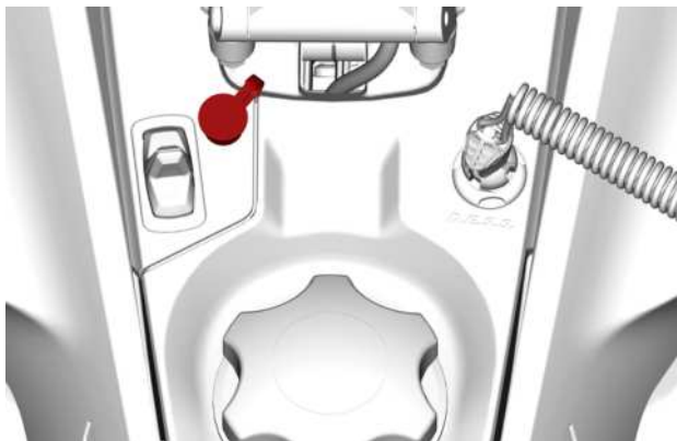
TYPICAL — DRIVER - ELECTRIC VISOR JACK CONNECTOR LOCATION
