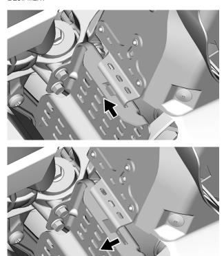
3. Insert belt guard tab between bottom pan and hook.
