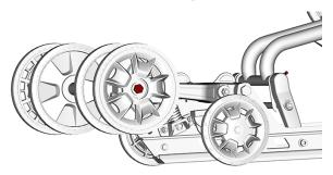
Tighten or loosen both adjustment screws to increase or decrease track tension.
