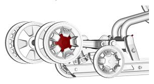
5. Loosen the rear idler wheels retaining screws.
