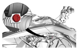
9. Remove the upper body module retaining screws on both sides.
