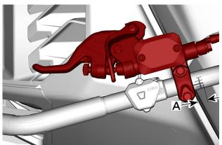
A. 0 to 9 mm (0 to 0.354 in) between the start of the handlebar mark and side of the brake lever
