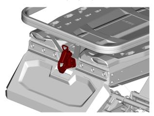
To open the hook, push and turn the handle to retract locking plate.
