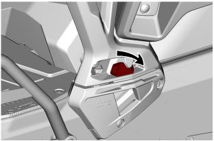
3. Pull the backrest upwards to remove..
