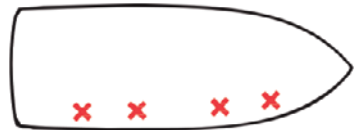
Improper (Starboard Heavy) KC-1340.1
