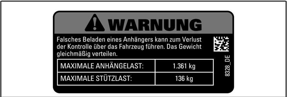
**Ziehen eines Anhängers – Warnschild**
