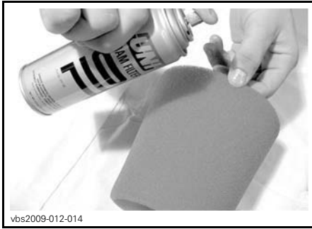
TYPICAL - OIL THE FOAM FILTER
