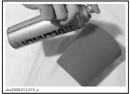
TYPICAL - SPRAY THE FOAM FILTER
