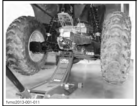
TYPICAL — BACK UP POINT LOCATION
