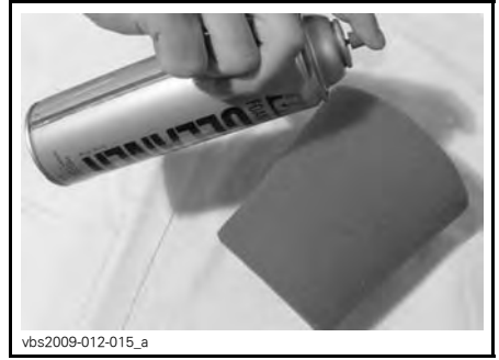
TYPICAL - SPRAY THE FOAM FILTER
