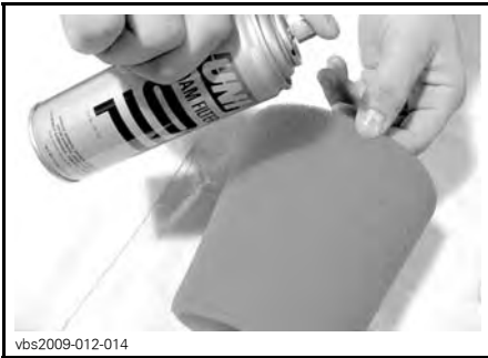
TYPICAL - OIL THE FOAM FILTER
