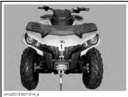
1. Front tie-down point location
