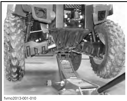
TYPICAL — FRONT UP POINT LOCATION
