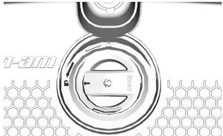
If the knob is hard to turn, install the provided molded handle over the knob to have a better grip. This molded handle is located on the wall of the compartment.
