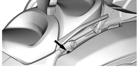
To activate or turn OFF the heating grip, press the button.
