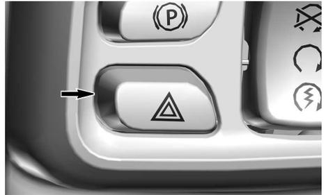
Push the button to turn ON the hazard warning lights.
