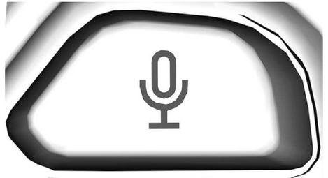
Used to trigger the voice assistant of the phone. The operator must have a phone and a headset connected via Bluetooth to use this function.
