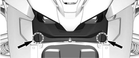
2. Pull the service cover forwards to remove it from the vehicle
