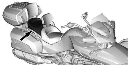
2. Slightly pull backrest forward to unlock it and lift to remove.
