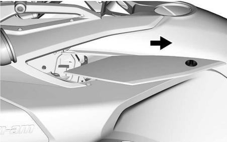
**TYPICAL****Installing the Lateral Service Cover**
