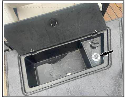
FLUSHING PORT — TYPICAL
