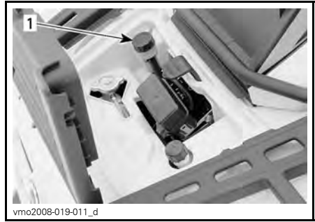
TYPICAL - SERVICE COMPARTMENT 1. Reservoir
