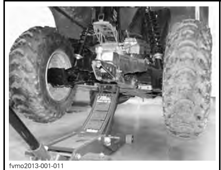
TYPICAL — BACK UP POINT LOCATION
