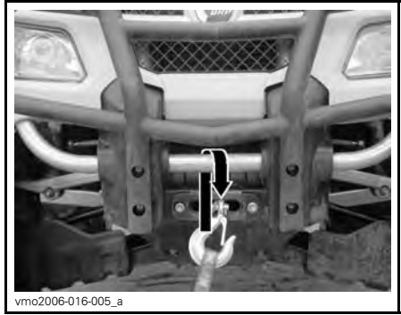
TYPICAL — FRONT TIE-DOWN POINT LOCATION
