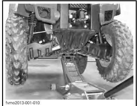
TYPICAL — FRONT UP POINT LOCATION
