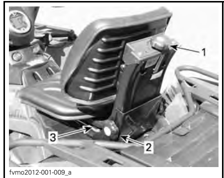
1. Seat suspension adjustment 2. Backrest height adjustment 3. Seat longitudinal adjustment
