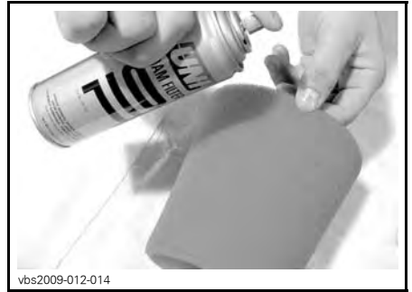
TYPICAL - OIL THE FOAM FILTER ELEMENT
