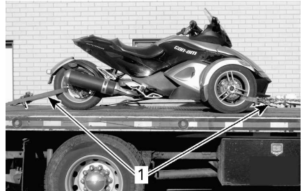
TYPICAL - VEHICLE FACING TOWARDS FRONT OF TOWING
