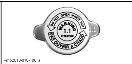
vmo2010-010-100_a LABEL 11 - LOCATED ON RADIATOR CAP
