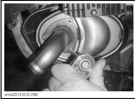
vmo2012-012-709 TYPICAL - REMOVE TAIL PIPE
