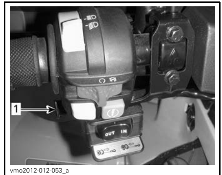
TYPICAL 1. Winch remote control connection
