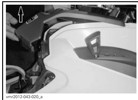
LIFT REAR PORTION
