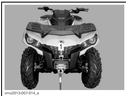
1. Front tie-down point location
