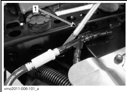
TYPICAL - CAREFULLY CUT HOSE
