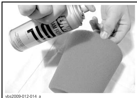
TYPICAL - OIL THE FOAM FILTER ELEMENT
