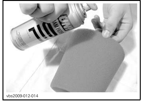
TYPICAL - OIL THE FOAM FILTER ELEMENT
