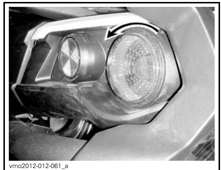
ROTATE TAILLIGHT CCW TO REMOVE
