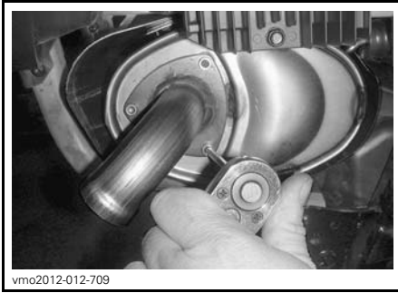
vmo2012-012-709 TYPICAL - REMOVE TAIL PIPE
