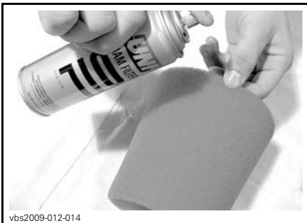
vbs2009-012-014 TYPICAL - OIL THE FOAM FILTER ELEMENT
