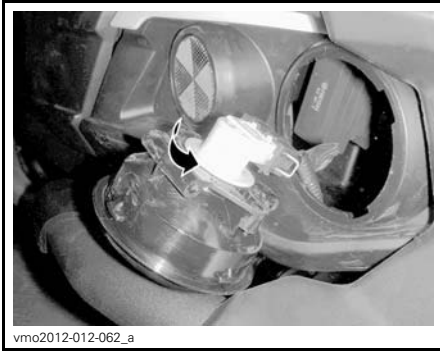
vmo2012-012-062_a ROTATE BULB COUNTERCLOCKWISE
