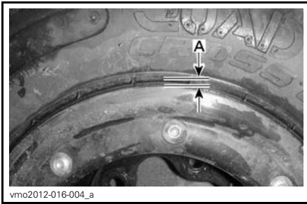
A. Gap (must be equal all around the wheel)
