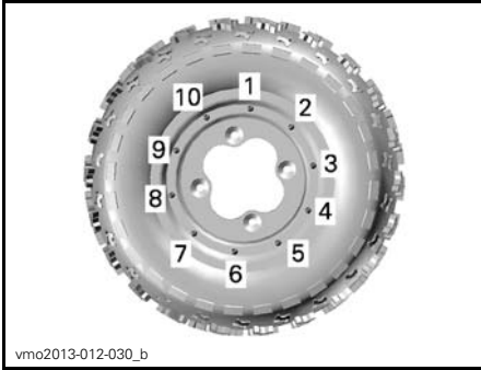
10-BOLT BEADLOCK WHEELS — FINAL STEP TIGHTENING SEQUENCE
