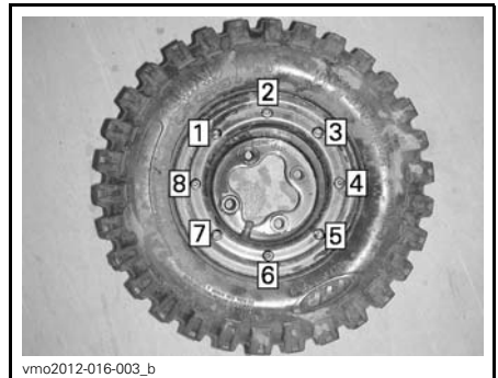
8-BOLT BEADLOCK WHEELS — FINAL STEP TIGHTENING SEQUENCE
