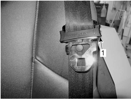
TYPICAL - LOCKED POSITION
