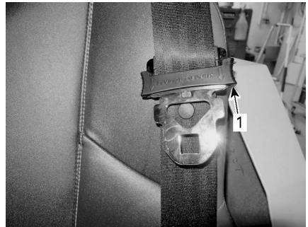
TYPICAL - LOCKED POSITION
