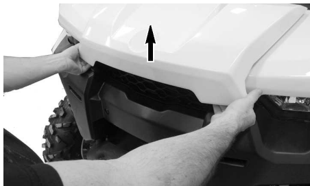
LIFTING FRONT SERVICE COVER EDGE.
