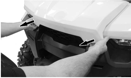
PULLING ON FRONT SERVICE COVER EDGE.
