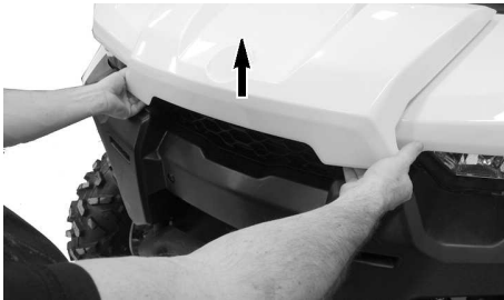
LIFTING FRONT SERVICE COVER EDGE.
