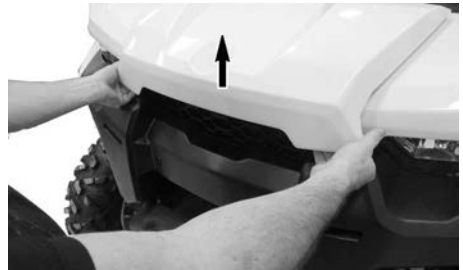
LIFTING FRONT SERVICE COVER EDGE.
