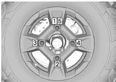
TIGHTENING SEQUENCE
