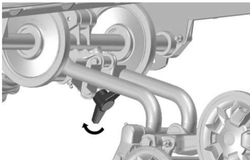
***RUOTARE LA MANIGLIA A FINE CORSA IN SENSO ORARIO -
