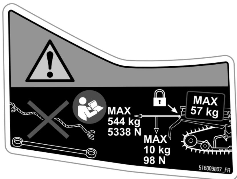
CHARGE CARGO MAXIMALE ET CAPACITÉ DE REMOR-
