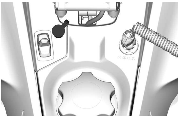
TYPICAL — DRIVER - ELECTRIC VISOR JACK CONNECTOR LOCATION
