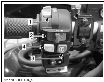
TYPICAL — MULTIFUNCTION SWITCH
