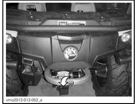
TYPICAL - REAR TIE-DOWN POINT LOCATION
