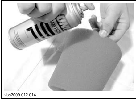
vbs2009-012-014 TYPICAL - OIL THE FOAM FILTER
