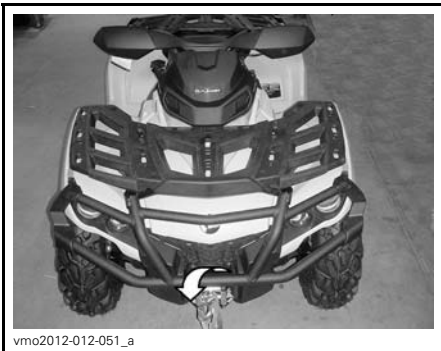
TYPICAL - FRONT TIE-DOWN POINT LOCATION
