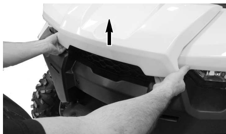
LIFTING FRONT SERVICE COVER EDGE.
