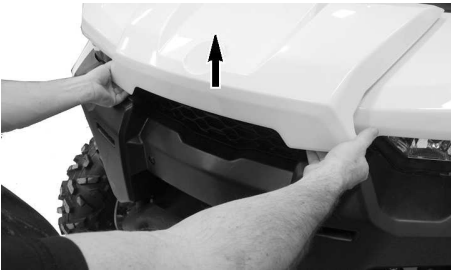
LIFTING FRONT SERVICE COVER EDGE.
